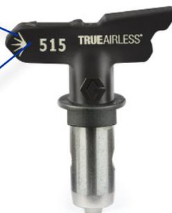
The orifice size defines the amount of paint that will flow through the tip. It is indicated by the last two digits: 15 in this case corresponds to a hole size of 0.015 of an inch or 0.38 mm. Your actual flow rate will depend on your spraying pressure and the paint you are using: high pressure - equals more flow; heavier paints equal less flow.
